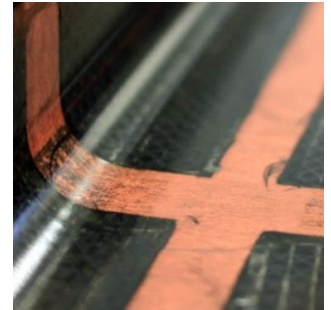
Embedded conductive path from INVENT GmbH.
